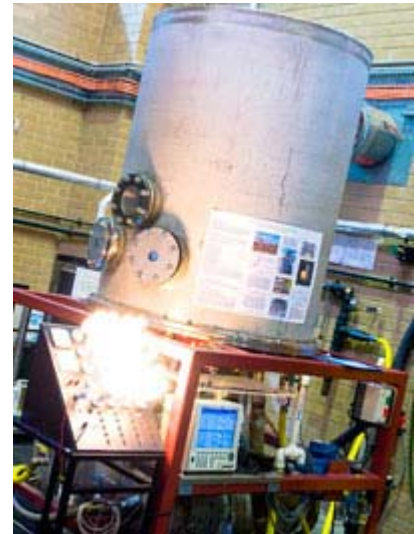
The dual geothermal system combines fresh water production with electricity generation.
